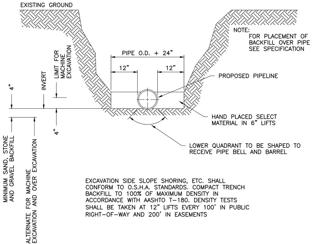
EXCAVATION SIDE SLOPE SHORING, ETC. SHALL CONFORM TO O.S.H.A. STANDARDS. COMPACT TRENCH BACKFILL TO 100% OF MAXIMUM DENSITY IN ACCORDANCE WITH AASHTO T-180. DENSITY TESTS SHALL BE TAKEN AT 12" LIFTS EVERY 100' IN PUBLIC RIGHT-OF-WAY AND 200' IN EASEMENTS
