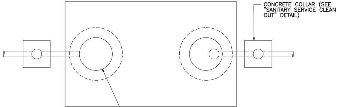
ADJUST WITH COURSE(S) OF BRICK AND MORTAR TO BRING TO GRADE (MIN. 2 COURSES OF BRICK - 6") (MAX. 5 COURSES OF BRICK - 18")
